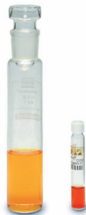
Comparison of the amount of chemicals used by the standard method and the cuvette test.
